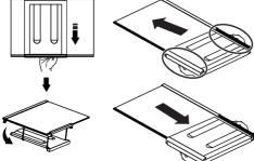
To group the wine rack, first remove the glass shelf from the refrigerator. Place it on the glass shelf by pushing the plastic part through the front and back grooves as shown in the picture. The product will be ready to use with the foldable wine rack.
